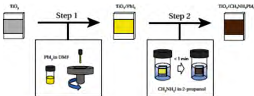
Fig. 12. Scheme that illustrates the deposition of the \text{CH}_3\text{NH}_3\text{PbI}_3 perovskite via sequential deposition technique. \text{PbI}_2 is first deposited via spin-coating (Step 1) and subsequently transformed into \text{CH}_3\text{NH}_3\text{PbI}_3 by dipping in solution of \text{CH}_3\text{NH}_3\text{I} (Step 2).
